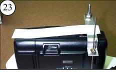
Lay the Brace on the camera. Trim one end if it overhangs the camera or the Shutter Arm.
