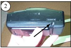
This camera has a tripod mounting hole in its base. If your camera doesn't have one, put pads of Velcro at the 4 corners of its base to attach it to the Camera Deck.
