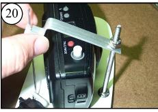
Center the Arm over the button. Press & hold for 15 seconds to bond the Button to the Arm.
