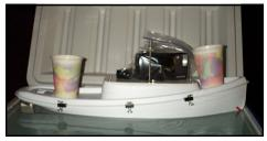
Set in water. Put two cups on deck as shown. Add weight to cups until you meet the waterline marks.
