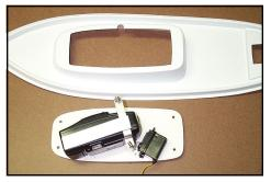
Mark 4 places on the Camera Deck 1/4 inch in from each corner and drill 3/16th inch holes through
