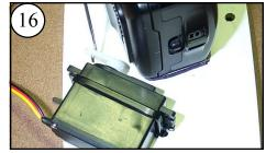
The attached servo will look like this from the top. The servo is in its "take photo" position. Set this by connecting
