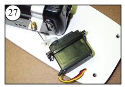
To insert the servo wire through the deck, drill two 1/8 inch holes 1/2 inch apart. Connect the holes with a hobby knife to make a slot.
