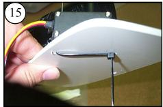
Attach the servo to the Camera Deck with one nylon Servo Tie. Make sure it is tight!
