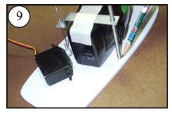
Drop the Shutter Arm Mounting Bolt strait through the Shutter Arm and mark the deck.
