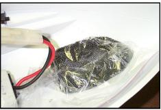
Combine the bow cup and bag ballast, mix with epoxy (in the bag), and press into the bow as shown.
