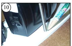
This camera has a sliding lens cover. I had to allow space for it to slide behind the Bolt.
