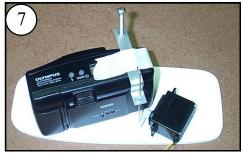
Orient the Servo to a position that allows it to pull the Pushrod strait down.
