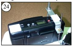
Attach Velcro to the camera and to the top of the Shutter Arm.
