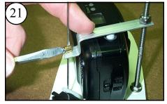
With the servo in the "take photo" position, push down on the Arm until the camera's shutter clicks. Tighten the Pushrod Keeper.
