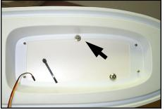
Underside of installed Cam Deck. I had to notch the opening to fit the Shutter Arm Mounting Bolt.
