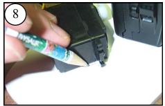
Mark the underside of the servo mounting flange on the deck.
