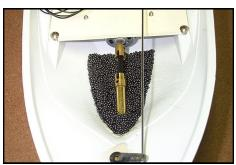
The stern ballast looks like this installed. Keep it away from the Motor-Shaft Coupling.
