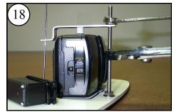
Grasp the Shutter Arm Mtg. Bolt with pliers at the center flat of the bolt. Tighten the Adjusting Nut with a 3/8 inch or 10 mm wrench until the Shutter Arm is level as shown.
