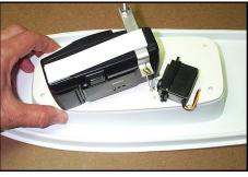
Set the Camera Deck on the Cabin. Mark the 4 holes on the Cabin with a pencil.
