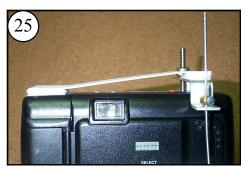
Place the Shutter Arm Brace as shown. This will keep the Shutter Arm centered in place.
