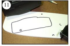
Outline the camera and add a mark for the tripod mounting hole of the camera on the Deck.
