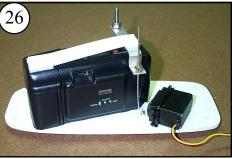
The servo arm should not strike the Deck when taking a photo. Adjust the Keeper so the servo travels just enough to click the shutter.
