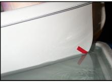
The bow waterline mark is in the center of the curve of the bow as shown by the red piece of tape.
