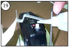
Put a droplet of CA glue on the top of the Shutter Button to glue it to the Shutter Arm. Don't glue the Button to the camera!
