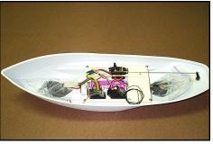
Put 8 ounces each of ballast weight into two plastic bags. Put them into bow and stern of the Hull.
