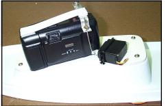
Attach the Camera Deck to the Cabin with 4 screws. Tighten gently until snug.
