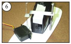
Tape the Shutter Arm to the camera, centered over the camera's shutter button.
