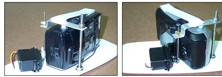
You are finished! Here are two examples of completed Camera Decks with standard servos. On the left is a 35mm camera shooting to a shallow right-front. On the right is a digital camera aiming left-front. To remove the camera, detach the Shutter Arm Brace, Raise the shutter servo to its highest position. Remove the Mounting Screw. Slide the camera
