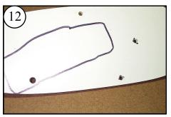
Drill a 1/4 inch hole for Camera Mounting Screw, 3/16 inch holes for the servo & Shutter Mtg. Bolt.
