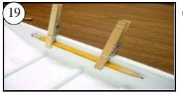
Set the Liner into the Hull stern-first to align the rear, then press into place. Hold for 1 minute. If necessary, you can clamp the sides as shown
