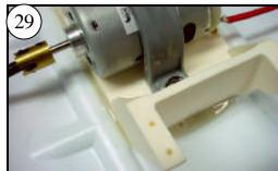
Apply filled epoxy to the underside of the Motor Mount. Set the Motor Assembly in place. Adjust to align the Motor Shaft to the Stern Tube. Let the excess epoxy flow out as shown.
