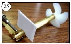
Install the Prop Shaft Coupling End onto the Prop Shaft. Make sure there is a 1mm space between the Coupling and the Stern Tube. 3 pieces of paper will make a good
