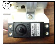
Compare your servo to the drill reference marks on the motor mount. Drill 1/16" holes for the servo screws.
