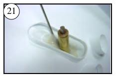
Tilt up the Stern Tube. Put filled epoxy on top and under the tube. Put just a little under it. Twist the Stern Tube to distribute.
