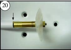
Insert the Stern Tube Assy into the hull. The mark should be just visible at the
