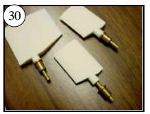
Slip the Rudder Bearings onto the Rudder and Flankers. Make sure they spin freely. If binding, check the shaft for plastic residue. **6**
