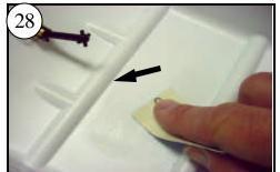
Scuff the mount area of the Hull Liner, and the underside of the Motor Mount with medium sandpaper for best adhesion. Sand the inner edges of the floor braces too.
