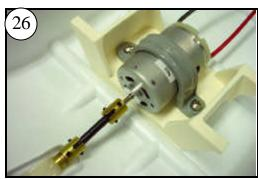
Test-fit the motor assembly. The dogbone should have about 1/16" of forward and backward play.
