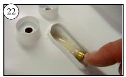
Press the Stern Tube down into position. Check the mark on the underside. Keep
