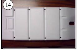
From the underside of the Hull Liner. drill 7/32" holes about 1/4 inch from each end of the four floor reinforcements. These will allow trapped moisture to dry.
