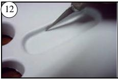
Use a hobby knife to score and cut the Stern Tube opening from the underside of the Hull Liner.
