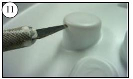
Cut off the caps of the 3 rudder molds. Cut just below the rounded top edge. Very thin plastic here. Use a new sharp blade.
