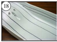
Clean any debris from the Hull. Using these lines as a reference, put 4 beads of medium CA on the floor, and 2 beads on each side of 5
