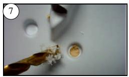
Use a sharp 1/4" drill bit. Use gentle pressure. The plastic is very thin. Keep bit centered in recess as you drill.
