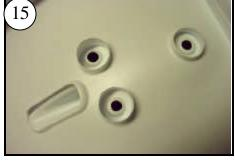
Test-fit the Liner into the hull. Push it rearward until it stops against the stern of the hull. The cups form molds for epoxy to secure the 3 rudder bearings.
