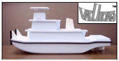
Length: 21.5 in. Beam: 6.5 in. Draft: 2 in. Displacement: 6 lbs.
