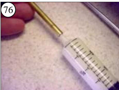
76 Fill the Stern Tube with your favorite lubricant. Greases seal well but can cause some drag on the motor. Thinner lubricants cause less drag but may need refilling more often.
