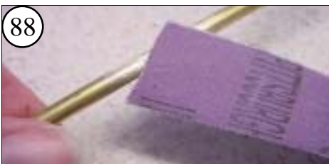
88 Clean off any grease residue and then scuff the Stern Tube so it will bond with the filled epoxy when installed. Sand the recesses for the Motor Base and the Stern Tube slot.
