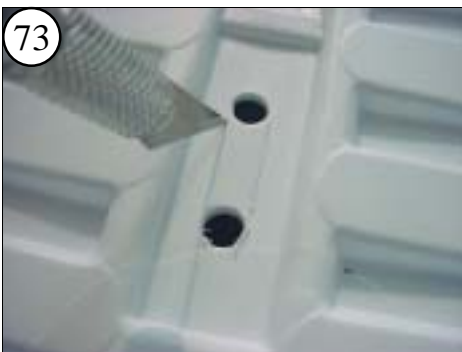
73 Score along the edge of the raised area with a hobby knife. Continue scoring straight down until you have connected the two holes.
