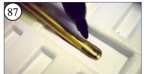
87 Mark the Stern Tube where it passes through the hull. This marks the area you will sand. From the Bow, check the alignment of the Prop Shaft to the Turn Fin. Slide the Motor Base left or right to center the Propeller.
