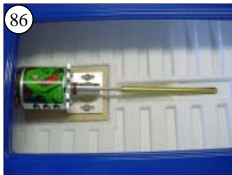
86 The motor base or prop shaft assembly should not bind to the hull. Adjust the motor mount screws or the length of the prop shaft to the Turn Fin. Slide the Motor Base left or right to center the slot in the hull to align the prop location.
