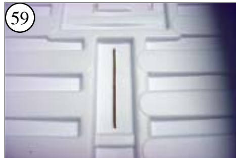
Repeat scoring both sides of the raised line until you are through the hull. Remove the strip of plastic at the center.
