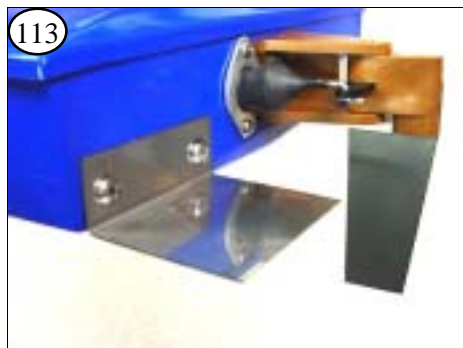
113 Trim Tabs are installed level with the bottom of the hull at the outer edges. Drill 1/16th inch holes to mount them. The oval holes in the Tabs will allow some adjustment after installing.
