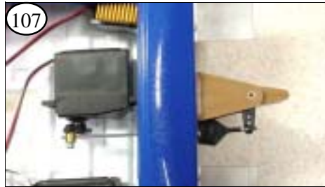
107 Connect the radio to "Center" the servo. Locate the Steering Servo so the Pushrod will be strait. The Servo Arm vertical and the Rudder Arm square.
