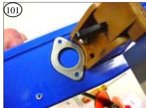
101 Temporarily install the rudder with 2 screws. Use the Bru-Line™ Pushrod Boot Bracket as a template to mark the centers for three holes needed.
