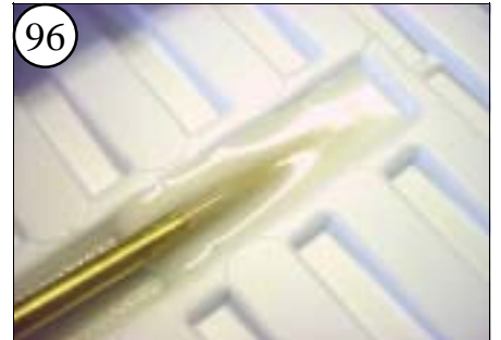
96 Fill the recess. Push epoxy under and on top of the stern tube. Before the epoxy cures, check the alignment.
