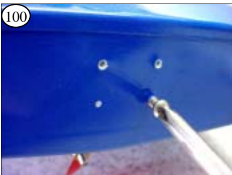
100 Use one of the rudder mounting screws to thread the holes for the rudder. Use some pressure to help the screw bite into the PVC reinforcement without causing the Hull to pull away.
