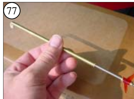
77 White lithium grease, or a synthetic grease works well. They can be thinned. Push out the excess grease by inserting the Drive Shaft. Clean any excess grease from the Stern Tube with solvent.
