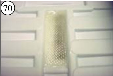
70 Press the fiberglass cloth into the epoxy until it is saturated. Check the alignment of the Turn Fin frequently until it cures.
