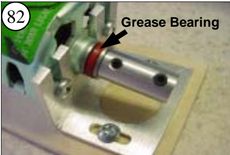
82 Install the 3-piece Thrust Bearing and the Coupling, adjusting so the coupling pushes against the bearing without binding.
