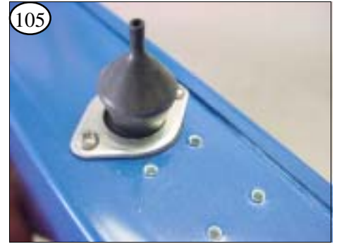
105 Install the pushrod boot to the transom. Make sure the boot is centered in the aluminum bracket.
