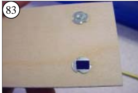
83 Put a tiny piece of electrical tape over the center of the T-Nuts to prevent epoxy from filling the threads.
