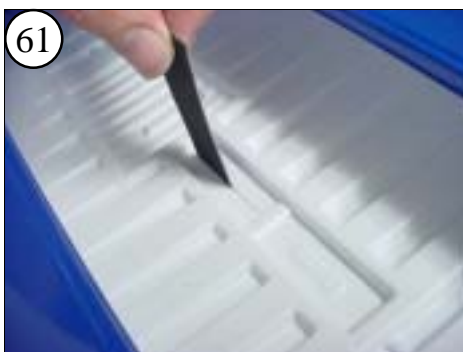
The Turn Fin must fit without binding. Use the strip of emery cloth to widen the slot as needed. Sand slowly and frequently check the fit.
