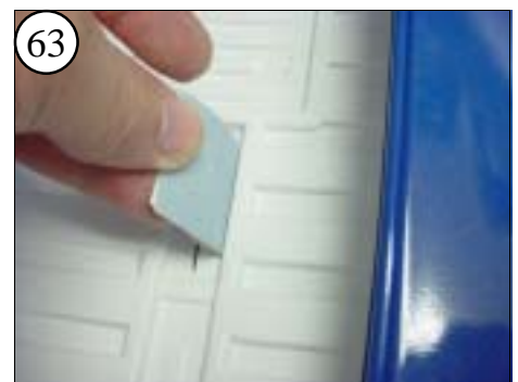
Don't forget to sand the walls of the recess as well. Same with the walls and ribs of the Motor recess and the pass-through for the Stern Tube.
