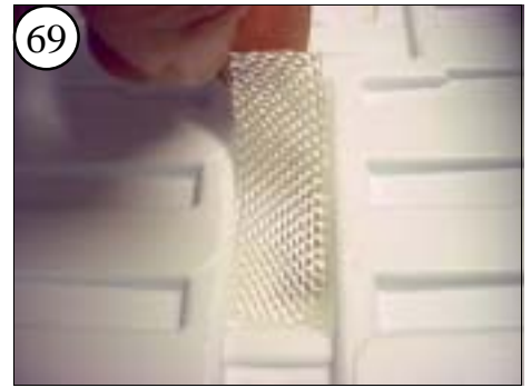
69 Reinforce the Turn Fin installation by laying a scrap of fiberglass cloth, or other material, into the epoxy.
