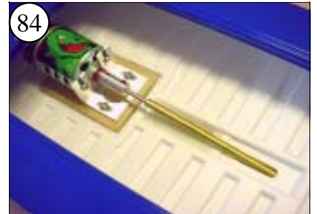
84 Install the Drive Dog, Prop, & Prop Nut, then slip the Stern Tube into the hull and attach fully into the Coupling.
