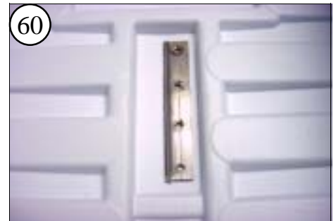
Test-fit the Turn Fin into the slot you just made.
