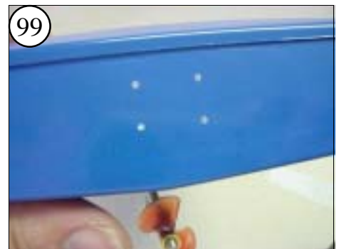
99 Use a push-pin to press marks through the template onto the transom. Drill four 1/16th inch holes at the pin marks on the transom.
