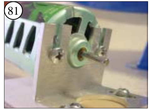
81 Install the motor with the M3 screws in the lowest position on the Mount. Lightly grease the Thrust Bearing.
