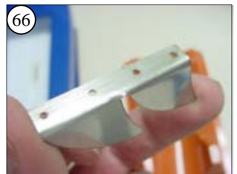
Scuff the flange of the Turn Fin on both sides with the emery cloth. Don't sand the blades of the Turn Fin.
