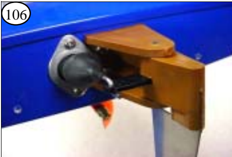
106 Put a little grease on the pushrod to help it slide into the boot, and install the rudder with 4 screws.
