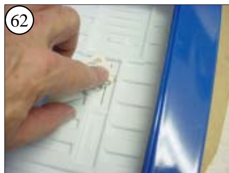
Sand the inside of the Turn Fin recess so the filled epoxy will bind it to the hull.
