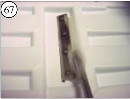
67 Hold the Turn Fin at an angle and push filled-epoxy under its flange until it appears behind the holes.
