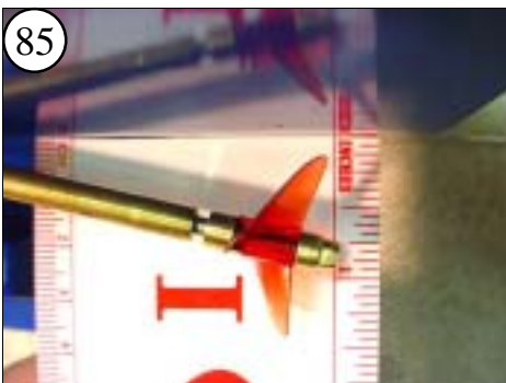
85 The prop should be spaced approximately 1/8 of an inch from the underside of the hull with a 1/8 inch gap between the drive dog and stern tube.
