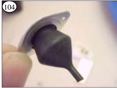
104 Insert the Pushrod Boot into its mount as shown.
