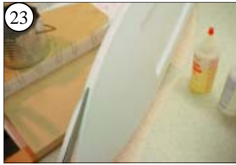
23 Clean your epoxy brush with alcohol. Cut out the Deck. Cut carefully as this cut edge will be visible on the finished boat.
