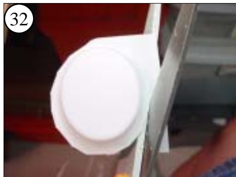
32 Rough-cut the Helmet Mount as shown. Cut close to the curve of the plastic.
