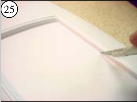
25 Use a Hobby Knife to score around the bottom of the hatch opening. Repeat this 2-3 times until you cut through. Scored styrene will snap apart when flexed.
