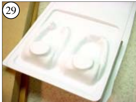
29 Then, carefully trim along the marked line. Sand the round corners smooth.
