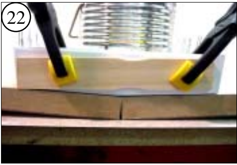
22 Make a final alignment check of the hull to be sure it is centered to the angle of the blocks on both ends.
