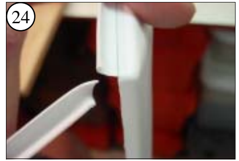
24 When you get to a corner, break away the scrap, then continue cutting. Sand the cut edge smooth.
