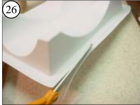
26 Trim the Boat Stand. After trimming, you can use sandpaper to smooth the edges or to remove any high spots along the cut.
