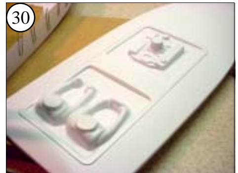
30 Test fit the Hatch to the Deck. Sand the hatch edges as needed to fit.
