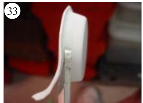
33 Then, trim away the bell leaving a strait slope to the side of the Mount.
