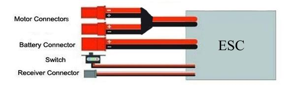
For twin-screw RC Destroyers, follow the color of the wires through the "Y" junction. As viewed from the rear, the left motor is wired normally, red wire to red wire through the "Y" junction and turns counter-clockwise. The right motor is reversed, red wire changes to black, and turns clockwise. Both motors are wired normally, red to "+" and black to "-" to their plug pigtails. This allows a correctly wired spare motor to be substituted for either side.
