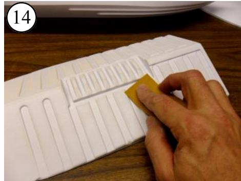
14 Sand the underside of the hull liner with the 100 grit sandpaper.
