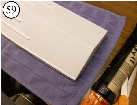
59 Set the hull into the deck transom-first with no gaps.
