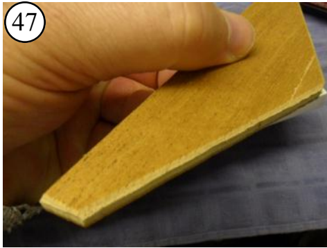
47 The side to glue to the transom is the side with beveled edges. Test fit before gluing.
