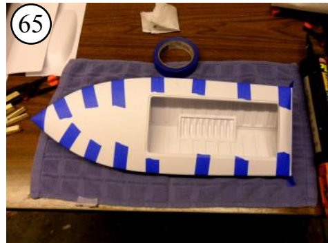
65 There are no strips of tape at the transom. The slope of the deck would cause the transom to roll in if pulled down.
