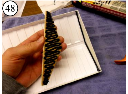
48 Apply sealant to the transom reinforcement and set into the transom.
