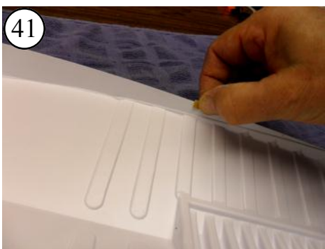
Do the same on the sides of the hull. This lets the sealant or glue grip the plastic.
