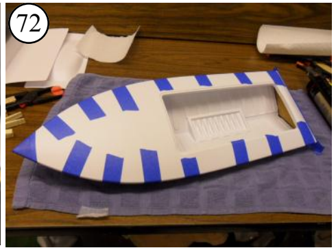
72 Check under the deck flange along the side making sure the tape wasn't
