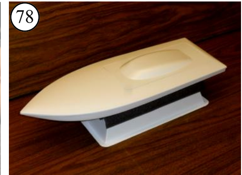
78 Trim the boat stand along the marked line and your boat hull is complete and ready for painting!
