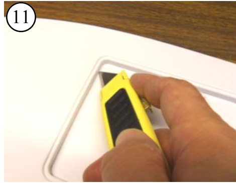
11 Score the hatch opening at the marked line 2 to 3 times until the opening separates from the hull.
