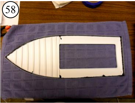
58 Set the deck with sealant on a padded surface.
