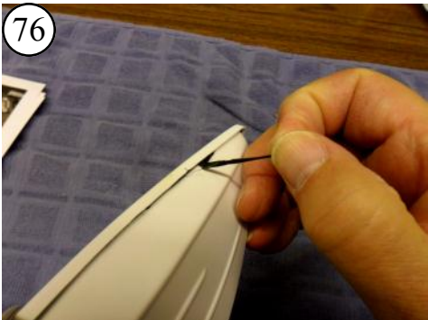
76 Now pull the sealant away from the hull. Sealant will not stick as well to an un-sanded surface.
