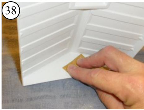
Sand where the transom reinforcement will bond to the hull.
