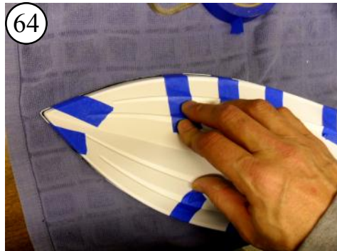
64 Continue taping every 3 inches or so toward the bow.
