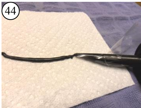
Keep experimenting until you have a good nozzle and can run a smooth bead of sealant.
