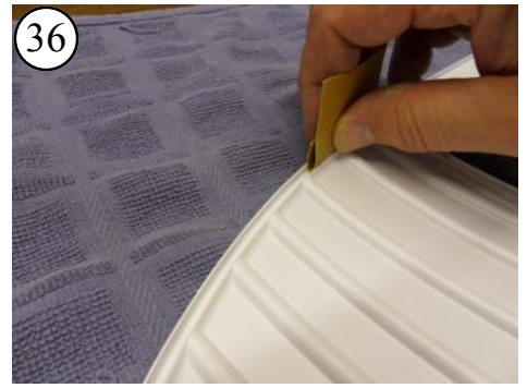
Fold a piece of sandpaper to sand the deck groove.
