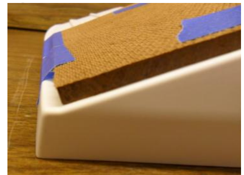
Close up of the edge of the scrap how it avoids the raised chine. Any smooth flat material will work here.
