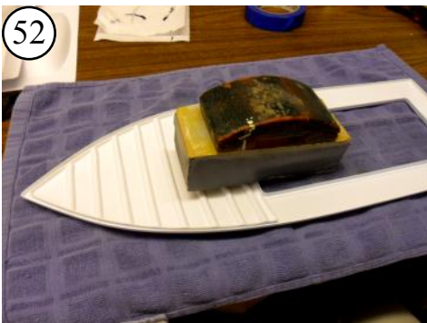
52 Set the deck upside-down on a towel and set a weight at the center to hold it
