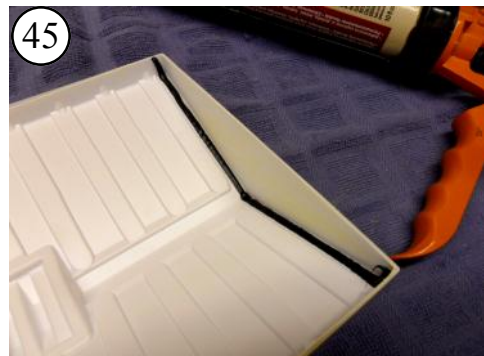
First, place a bead of sealant in the bottom groove at the transom for the transom reinforcement.
