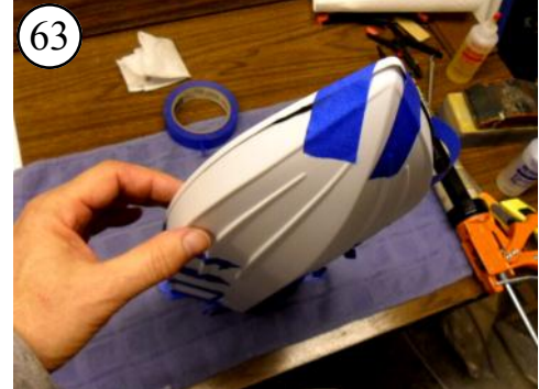
63 With pieces of tape ready, pull the deck over the hull and secure the bow as shown. Don't worry about sealant squeezing out.
