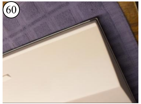
60 See that the sides fit inside the deck flange.
