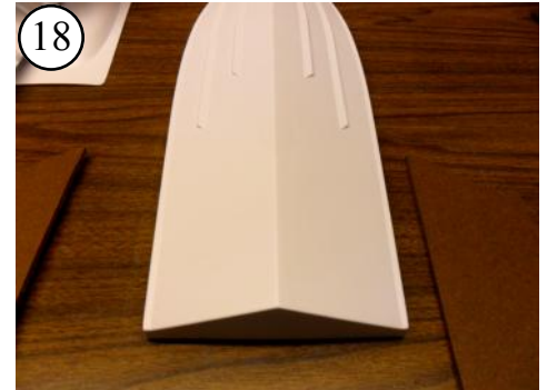
18 When gluing the hull liner, you want to clamp it firmly to the deck, but you don't want to clamp over the strakes or chines. (raised areas)
