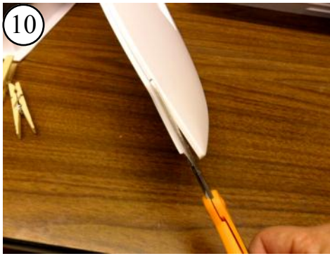
10 Cut slowly. The plastic is thicker on the deck than the hull.
