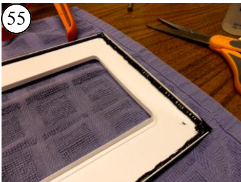
55 On the rest of the deck, fill the inside of the corner of the flange with a triangular cross-section. Put a thicker bead at the rear to reach the transom.
