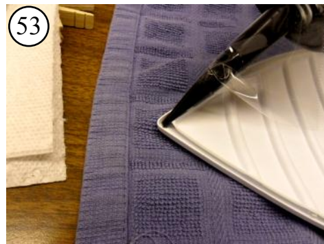
53 Start at the bow by filling the groove about 2/3 full of sealant.
