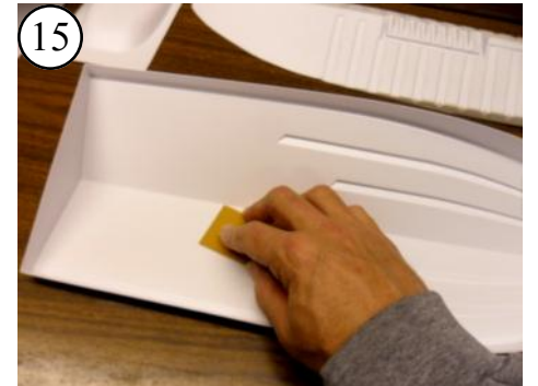
15 Sand the inside of the hull. Sand both in at least two directions for a better bond.
