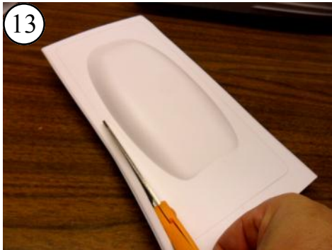
13 Cut the hatch on the marked trim line.
