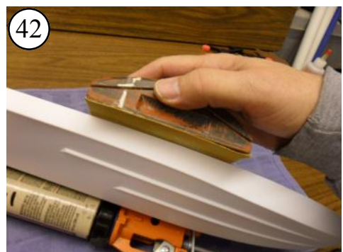
Check the edge of the hull and sand-level any uneven areas for a good even contact with the deck.
