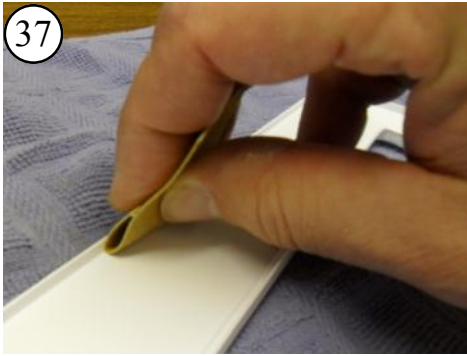
Sand the rest of the underside edges of the deck.
