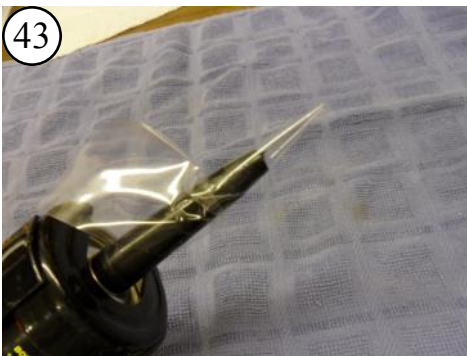
If you are using a caulking tube of sealant, make a narrower nozzle by wrapping the end with packing tape to a point and trim the tip for a 1/8" bead.
