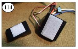
Cut the fuzzy "loop" side of the Hook & Loop fastener and put on the back of the Receiver and the Electronic Speed Control. 13
