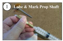
Squeeze the synthetic grease into the Stern Tube until it comes out the other end.
