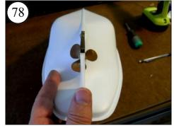
The Skeg and Rudder should align close to this. It does not have to be exact.
