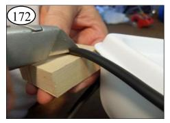
Continue the cut over the wood block or table. Hold it carefully to ensure a straight cut. Repeat for the other end.
