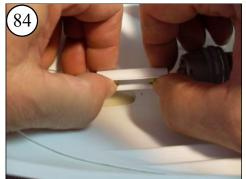
Set the Motor Assembly in place and clip each Coupling End into the Alignment Clip.
