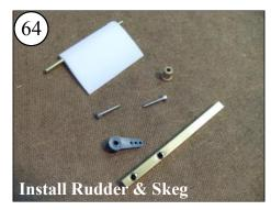
Open the Rudder Package. Take the brass Skeg and 2 screws.
