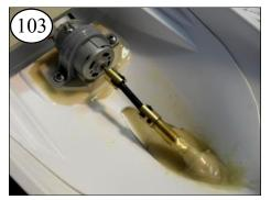
Set the Motor Assembly into the Liner. Insert the Dogbone between the Coupling Ends.
