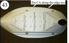
If using CA, these lines mark where you should put CA glue on the Internal Tray before inserting it into the Hull.
