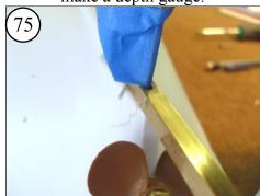
Drill until your "Depth Gauge" contacts the Skeg. You should pull out the drill once or twice during the drilling to remove plastic from the drill bit.
