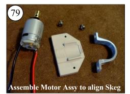
Unpack the Motor Package. You can install the 3/32 in. Coupling End to the motor shaft.
