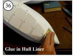
Turn over the Hull Liner and sand the areas that will contact the Hull.
