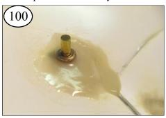
Mix the last batch of filled epoxy. Make sure the third layer is still lower than the top of the bearing.
