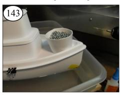
The bow should set just below your mark. The stern, about 1/8" below the top of the rudder.
