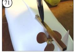
Mark the 2nd hole then loosen the first screw 2-3 turns.
