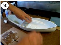
Press into place. If the sides of the Hull are not making good contact with the sides of the Liner, add rubber bands.
