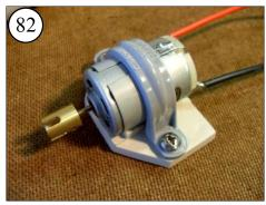
Set the motor into the tray just as shown. Screw on Motor Clamp & tighten the screws.
