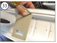
Instead of waiting for the CA to bond, go ahead and install the tray and screws. The screws will hold the strips in place.
