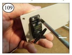
the Servo is oriented into the tray as shown.
