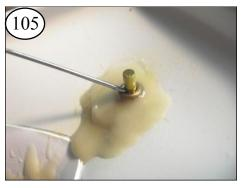
Use a paper clip or wire to put a droplet of oil on the rudder bearing at the shaft.
