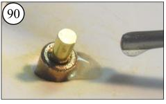
Put a couple of drops of the epoxy at the sides of the rudder bearing. Help it run around the bearing. Keep the epoxy off of the top of the bearing. 11
