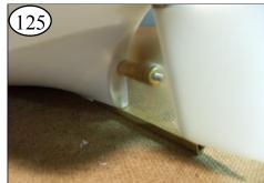
Check the direction of the prop. Going forward, it should be turning counterclockwise as seen from the back.
