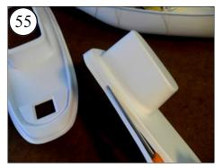
Cut curves by taking shorter snips. If the edge is uneven, you can sand the cut edge.
