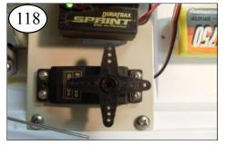
Fix this by removing the servo horn and rotating it to each arm until you find one that leaves the arm square to the servo body.
