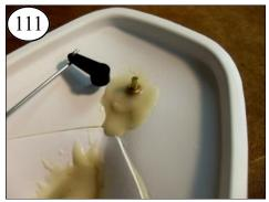
Put the Rudder Arm on the Pushrod like this, with the rod inserted from under the arm.
