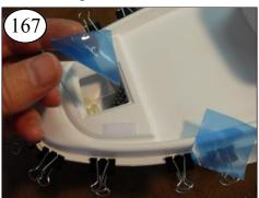
While you are waiting on the Deck/ Hull joint to cure, tape the rear hatch in place.
