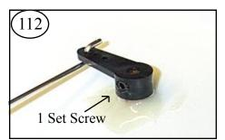
Press the Rudder Arm onto the Rudder Shaft. Align the rudder and tighten one set screw against the flat on the Rudder Shaft.
