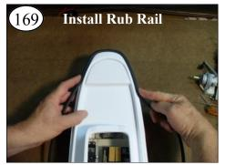
Engage the center of the Rub Rail on the Stern. Without pulling hard, run it toward the bow on each side.
