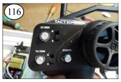
Connect the ESC, battery, & servos from the instructions for your electronics. Set transmitter steering. adjustments to neutral.
