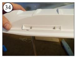
The screws should pull the Reinforcing Strip tight against the Hull Liner.
