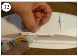
Apply Medium CA (super glue) to one strip. Hold the strip against the underside of the rail with the holes aligned.
