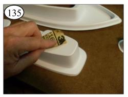
Sand the top of the Pilot House and underside of the Pilot House Roof. Glue together with CA.
