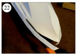
Trim the edges of the Hull Liner along the marked line.
