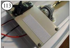
To align the Servo, we need to install the electronics. Hook-side of Hook & Loop is stuck to the Servo Tray.
