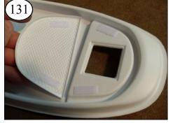
Remove the Hatch Cover and press the strips to set the adhesive.
