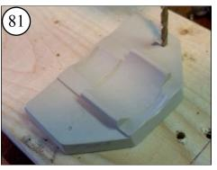
Drill two 7/64 inch holes into the marked dimples of the motor base.
