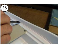
Set the Hull Liner into the Hull. Use a pencil to lightly mark the hull along the top of the Liner.
