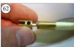
Insert the Stern Tube Assembly into the hull. Slide the 1/8 in Coupling End onto the shaft. Note the location of the flat on the shaft.
