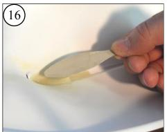
Set the reinforcement into the stern of the hull.
