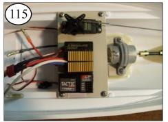
Attach the ESC and the Receiver to the tray. The servo is channel 1, the ESC is channel 2.
