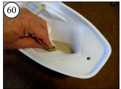
Sand all around the ballast and shaft area.
