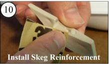
Sand all surfaces of the Skeg Reinforcement. The skeg is the square brass tube that supports the bottom of the rudder.
