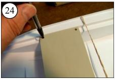
With the Servo Tray slid against the raised bumps on the liner, mark the 4 holes with a pencil.
