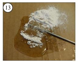
After mixing, fold in the same volume of filler material. I'm using Talcum Powder. The filler makes the epoxy less brittle after it cures.
