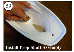
Sand the area where the motor and motor mount will be glued.
