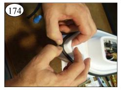
Hold tight for one minute. Check under the glued ends and if not together, hold that spot too. 18
