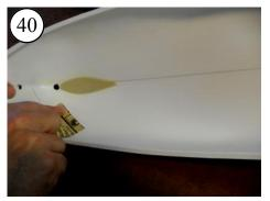
Sand the area inside the Hull below the marked line. Sand the areas around the rudder and prop shaft holes.
