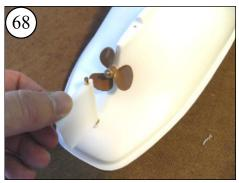
Insert the longer brass rod of the rudder into the bearing.
