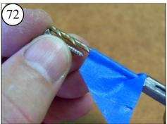
Using a Skeg screw as a guide, wrap a piece of tape on the drill to make a depth gauge.
