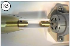
Note the orientation of the Coupling Ends in the Alignment Clip. If needed, pull the ends out a little and rotate them so they contact the clip as shown.
