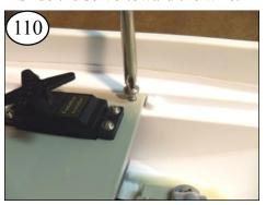
Install the 4 servo screws. Make sure Re-install the Servo Tray. The stern of the boat is on the right in this photo.
