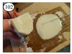
Put epoxy on the bottom of the Motor Mount.
