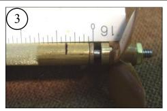
Put a mark on the Stern Tube about  $3/8^{ths}$  of an inch from the end of the bearing.
