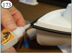
Apply a little CA to one end. Using the Deck/Hull flange as a guide, roll the ends together and hold.
