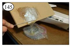
Pour front ballast bb's into a plastic bag. Mix 2 one-inch circles of epoxy parts A & B and add to the bag. Use NO FILLER with this epoxy.
