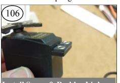
Install Servo & Rudder Linkage
