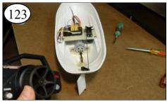
Turn the wheel of your transmitter to see if the rudder works. This is a LEFT turn of the wheel. If the rudder is opposite, then reverse the transmitter steering switch.
