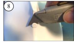
With a rocking motion, slice through the Stern Tube hole as shown. Cut down 2/3rds then cut up 1/3rd to complete.
