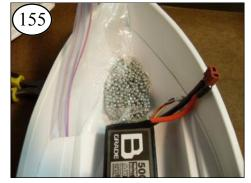
Remove the Coupling cover. While the epoxy is still wet, check the arrangement of the front ballast.
