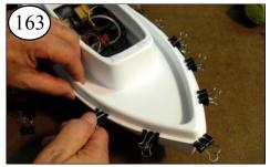
Align the bow-center and clamp. Then, work rearward left and right aligning the outside edges of the Hull and Deck flanges as you go.
