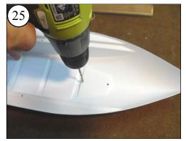
Drill 1/8 inch vent holes into the liner on each side of the floor ribs as shown.
