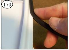
This bend will help the Rub Rail open and engage the flange of the hull. No need to glue it. It will stay in place.
