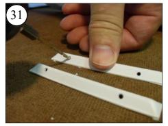
Drill the Reinforcing Strips as marked with a 3/32" drill.
