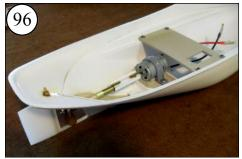
Let this first coat of epoxy "gel" (firm but not completely cured). We will apply 2 more coats in the next steps.
