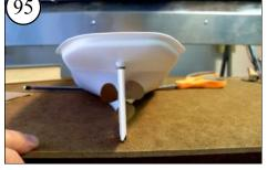
Check the shaft alignment. Confirm the motor is still centered and the mark on the side of the Prop Shaft is still aligned.
