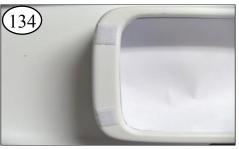
Stick the Hook & Loop squares on the front and rear of the Cabin as shown. Peel tape. Set Pilot House on Cabin to adhere the Loop to the Pilot house. Remove Pilot House and press the Hook & Loop to set the adhesive.
