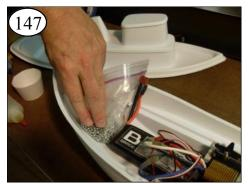
Still in the bag, press the ballast to shape it into the hull forming a flat topped triangle.
