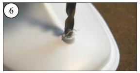
With a 1/4" drill bit, drill through the Rudder Bearing hole. Use gentle pressure. Let the drill slowly drill through the plastic to avoid it splitting.
