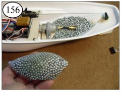
After it is fully cured, overnight, remove the plastic bag from the front ballast.
