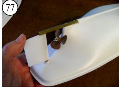
The Rudder should turn freely without binding.
