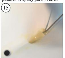
Put lots of filled epoxy in the recess of the hull where the skeg reinforcement will set.
