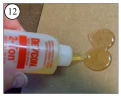
Measure out two inch-wide puddles of epoxy parts A & B.
