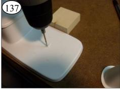
Drill a small vent hole in the center of the marked area.
