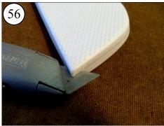
Sharp corners should be started with a razor using a rocking motion until the blade cuts into the plastic.
