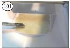
Put filled epoxy into the liner where the Motor will sit. If the Servo Tray is in your way, remove it.
