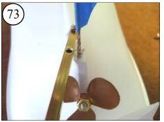
Rotate the Skeg aside, and drill only into the white plastic, not into the reinforcement yet.
