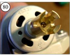
The end of the motor shaft should be flush with the bottom of the Coupling.
