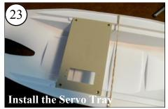
Set the Servo Tray into the Hull Liner as shown. If needed, use 2 rubber bands to snug the liner.
