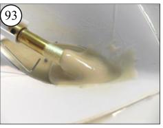
Put the filled epoxy over the Prop Shaft Assembly where it comes through the Hull.
