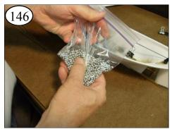
Knead the bb's with the epoxy until they are evenly coated. Set the bag in the bow of the Hull.
