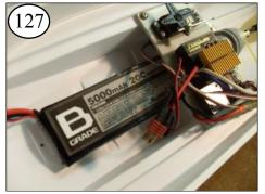
I tested with a smaller battery. To ballast the boat, I install the battery I plan to run in the boat.
