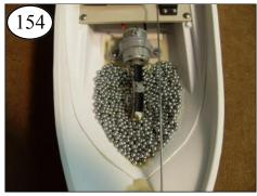
Arrange the ballast evenly on each side, with a open gap under the Coupling and Prop Shaft end.
