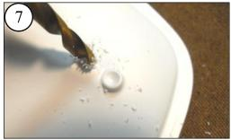
As you drill, check the alignment to ensure the hole is in the center.
