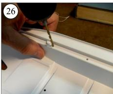
Drill 3/32 inch holes at the 4 marked Servo Tray holes.
