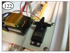
Now is the time for an Operational Check. Turn on the Transmitter, THEN the Receiver.
