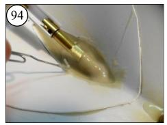
Push the epoxy under the Prop Shaft Assembly to eliminate any air bubbles under it.
