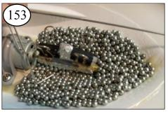
Arrange the ballast with a paper clip with a bend at the end to reach under the Coupling and Prop Shaft .
