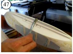
Dab along the sharp edges. 30minute epoxy can gel in 10 min.
