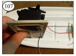
Insert the bottom wired end of the servo into the trav first as shown. Slide the servo toward the wire.
