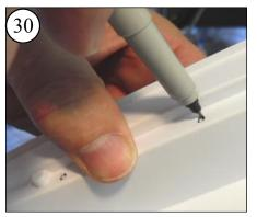
Mark the Reinforcing Strip through the Hull Liner.
