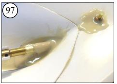
Mix a smaller batch of filled epoxy. Carefully apply a layer around the rudder bearing & put the rest over the Prop Shaft Assembly as shown.
