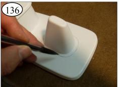
Center the Stack on the deck of the Pilot House. Lightly mark the location in pencil.
