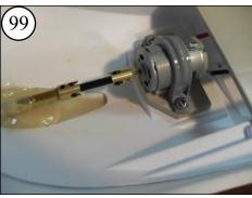
Test-Fit the motor to the Stern Tube with the Dogbone between the Coupling Ends.
