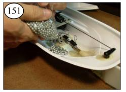
Cut the corner of the bag and squeeze the ballast into the stern.
