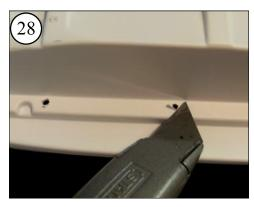
Trim any bits from the underside of the drilled holes.
