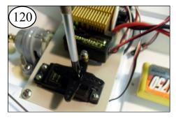
Return the servo horn to the servo. Install the servo horn screw. Slide the Rudder Pushrod into the hole of the E-Z Connector.
