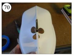
Align the Skeg with the Keel of the Hull.
