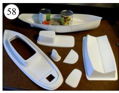
All trimmed. The hull should be set by now. Check the mixing board to make sure.
