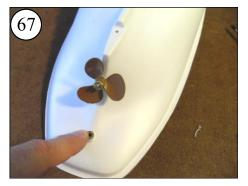
Press the Rudder Bearing into the 1/4 inch hole.
