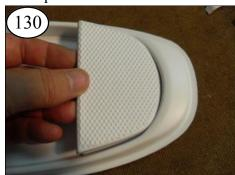
Align and press the hatch in place. This will cause the loop side to stick to the hatch.
