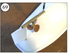
Slip the Skeg onto the rudder and attach the bow-end screw into the Skeg. Just snug the screw for now.
