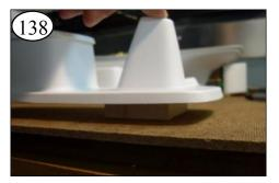
Lightly sand the underside of the stack and apply CA. Press 40 seconds onto the Pilot House deck supported by the wood block. 15
