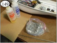
Mix two 1-1/2 inch circles of epoxy with no filler. The rear ballast is a often a little larger than the front.
