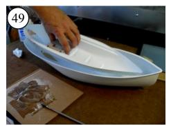
Insert bow-first, trying to avoid touching the sides of the Hull with the Hull Liner.
