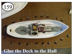
Arrange the 20 clips around the Hull evenly. Practice clamping the Deck to the Hull. Start at the bow and...
