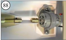
Rotate the Prop so see if the shafts appear to be aligned. Center the Motor Mount between the raised side ridges of the Liner.
