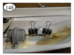
Clamp the 2 inch x 3 inch plastic bag around the Coupling and Stern Tube to keep out epoxy.
