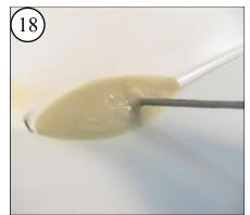
Cover the reinforcement with the squeezed-out epoxy. 5
