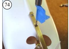
Align the Skeg and tighten the front screw. Now continue drilling into the reinforcement, using the hole in the Skeg as a guide to keep your drill centered.
