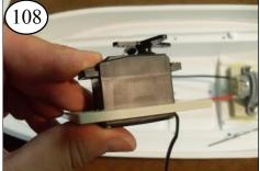
Push down on the other end and the Servo should snap into the hole. You may have to wiggle the servo a bit
