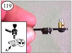
Install the E-Z Connector onto the 3rd hole from the center of the servo arm as shown.
