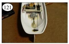
Align the rudder as shown. Now, tighten the screw on the E-Z Connector while holding the pushrod next to it. Any further adjustments can be made with the transmitter.
