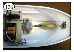
The Rudder Arm and the Servo Horn should be parallel to each other as shown. 14
