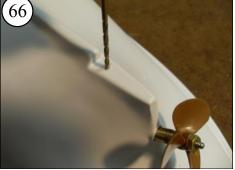
Use a 3/32 inch drill to drill a straight hole through the Hull 9 and Skeg Reinforcement.
