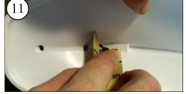
Sand the area inside the Hull at the stern to help the epoxy bond the skeg reinforcement to the Hull. Test fit the skeg reinforcement into the hull.
