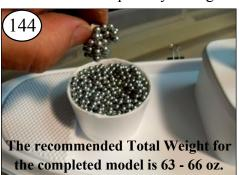
Use a small magnet or spoon to remove or adjust the ballast. To little is easier to fix than too much.
