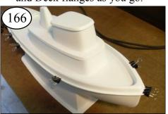
Notice the clamps are not jammed against the hull. They are centered on the flange. A few final clamps may need to stay on longer to bond.
