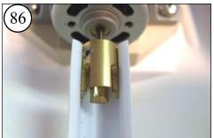
This lets the Alignment Clip make the best side contact with the Coupling End. Repeat pressing the Coupling Ends into the Clip shown in step 84.
