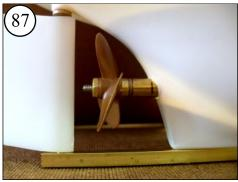
Check the mark on the Stern Tube. 3/8 inch from the end of the shaft bearing. It should look like this.
