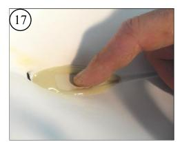
Press the Skeg Reinforcement into the epoxy.
