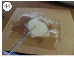
Mix the epoxy and add filler. Find the Epoxy Brush.
