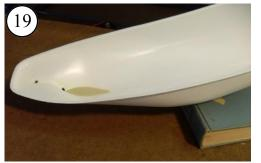
Tilt up the hull with a book to keep the epoxy in place as it cures.
