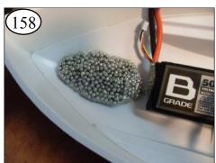
Peel off the paper tape and stick the ballast into the bow. It can now be removed easier to adjust its weight.
