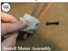
Once the epoxy cures, carefully slide off the motor and Alignment Clip. Sand the bottom and bottom edges of the Motor Mount.
