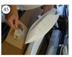
Holding the Liner, apply the epoxy by lightly dabbing the sanded areas.
