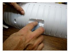
This is the correct Crossmember shelf insert for this side. It fits flush and evenly into the opening. The anchor points inserts fit any anchor point. Sand the insides of the two shelves and two inserts you marked.
