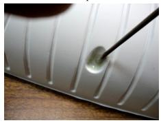
Fold-in an equal volume of filler powder & mix well. Scoop up some and distribute around the inside of the chosen anchor point. The insert is form-fit so little epoxy is needed.
