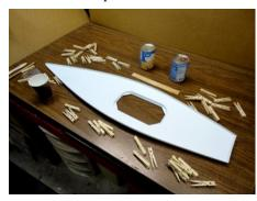
Attach 4 clothespins at the bow clamped to the 2nd & 3rd rib, then put one on the end clamped flat to the tip of both the Deck and the Deck Liner. The end pairs of clothes pins (yellow arrows) will be touching the deck evenly to ensure that there is no twist in the deck before the epoxy cures. Practice is over. Lay out the rest of your materials to laminate the Deck.
