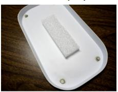
As they bite into the fiberglass backers, use a bent wire or Allen wrench for the leverage to screw them the rest of the way until they contact the washers. Don't forget to glue a piece of foam inside your Cockpit Cover. It will sink without some flotation.
