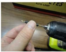
Remove the Crossmember. These holes will be drilled with a 3/32-inch drill. Insert the drill bit into your drill and slip the rubber hose depth gauge over it.
