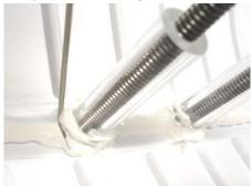
Remove the Crossmember, Keel Tubes & Keel Shoe. Install the two keel tubes. Put a bead of sealant along the center of the hull at the Keel Shoe outline. Just a 3/16" bead but put more around the grooves of each of the tubes. Use a bent wire to work the sealant into the grooves filling them. **Important** to get the sealant completely around the grooved part of the two acrylic tubes. This will form a seal between the tubes, the shoe and the hull so the
