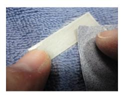
Sand the underside of the King Post Upper Mount. Sand inside the Transom inside the raised rectangle where the Transom Backer will be glued. Sand one side of the shorter fiberglass backer. Sand both sides of the white plastic spacer and the backer for the Mast Step. The short backer is for the Transom.
