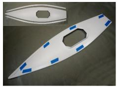
**Lightly score around the inside of the cockpit opening from the top of the deck.** Repeat until the center pushes out. **Score the deck reinforcing liner from its <u>underside</u>**. This leaves a raised lip around the top of the liner's opening. Set the scraps aside for testing paint or practice drilling holes. Tape the temporary deck clamping strips on top of the deck, even with the deck's edges.
