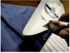
The tongue-in-groove joint will go together easier if the sharp edges of the plastic are reduced. Use your knife to lightly scrape only once or twice along both sides of the Deck groove and both sides of the Hull edge with the blade at an angle to the edge. Next you will insert the Hull into the Deck **without glue or sealant** to mark the sides of the Hull.
