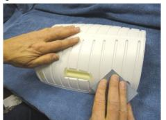
Sand inside the Hull at the transom back and sides. Carefully support the back of the transom while sanding as it is very thin. Sand the outside of the Transom Reinforcement. If the reinforcement epoxy is cured, sand the Hull Liner as shown.
