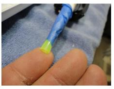
Lightly round just the sharp edge of the spout at the end of the caulking tube. Push the slit-end of the straw onto the caulking tube just past the end of the slits. Carefully tape to leave no gaps for the sealant to ooze out. Pinch the end of the straw to make it flat so it can slide into the Deck groove. If it comes out of the groove while you are applying sealant, take a paper towel and pinch it again to help it go back into the groove.
