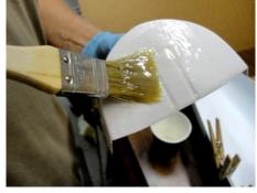
You will notice that in between the clothespins there may be gaps between the Hull and the Hull Liner. Clamp these gaps with another clothespin, not clamping the rib this time. Look for any epoxy oozing out of the top and clean it while it is still uncured. Apply the filled epoxy to the Transom Reinforcement.
