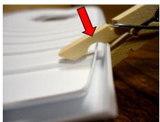
Take a clothespin and clamp the rib of the Deck Liner to the Deck near the Transom. Adjust it until the corner of the deck clamping strip falls into the notch of the clothespin. The flange of the Deck Liner is within the other notch in the clothespin. 5
