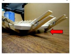
Put a 15 ounce can on the center stick then set the other two cans of vegetables on each end of the long stick as shown. At the stern, place two clothes pins on the end of the deck resting on the ends of the clamping strips. These clothes pins will touch the table and hold the stern-end of the deck assembly square to the build table.
