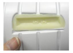
Press the insert into the epoxied recess. Wipe away any excess epoxy. Repeat for the other anchor point and the two Crossmember shelf inserts.
