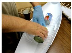
While holding the side together a little, set the Hull Liner into the hull and align it using the two locator bumps and the marked end lines. When you are confident it is in the proper place, set two 15 ounce cans of vegetables into the Hull Liner as shown.
