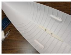
Use a Sharpie marker to plainly mark the 1/4-inch part of the drill. Drill the two dimples to 1/4-inch diameter. Turn the Hull over and set the Keel Mount Shoe into the hull.
