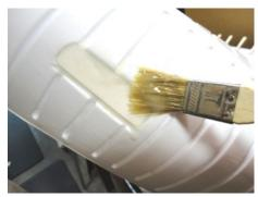
Mix 1-Pump of West Systems Epoxy and add 1 level tablespoon of filler. Brush onto the Hull Liner like you did the Deck Liner. When you are done, a little extra around the crossmember inserts will help strengthen this area. **Don't use all of the epoxy. Save some for the Transom Reinforcement.**
