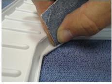
**Hazard:** Rare earth magnets are plated with Tin, Chromium, Cadmium or other harmful metals. Avoid dust and debris from scuffing them. Sand them outside. Take the row of magnets and sand one end to roughen the surface. Take a magnet from the other end and snap it over the sanded magnet. Repeat until **one side** of each magnet is scuffed. Sand the **underside** of each corner shelf of the Cockpit Opening.
