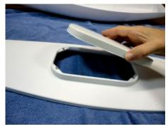
Turn over the deck. Now those four magnets are sanded-side-up and located right on top of the other magnets. You have already sanded the inside corners of the Cockpit Cover. Put a droplet of CA (Super Glue) on the center of each magnet.
