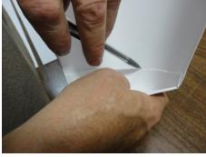
Carefully trim off the marked top of the Transom Reinforcement by scoring with a knife or use scissors. If scoring, lightly score once then repeat until you can break off the scrap. Set the Transom Reinforcement back into the transom firmly seated in place and mark the edges in the Hull for sanding.
