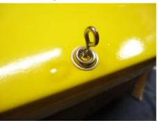
The stainless steel flanged finish washers help support the screw eyes from side loads. Start the screw eyes by hand.
