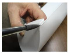
Set the Transom Reinforcement into the Transom end of the Hull and align to the sides of the hull. Mark along the Transom top and Hull Sides for trimming. Be careful not to move or shift the reinforcement while marking.
