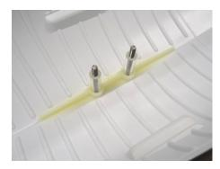
Set the Keel Shoe into the hull centered on the keel holes and mark the shoe's outline. Sand the underside of the shoe and sand the shoe's outline in the hull. Set the hull onto the Keel. Place the Keel Mount Tubes over the Keel Bolts with the end that is grooved on the bottom (arrow). Set the Keel Mount Shoe over the two tubes.
