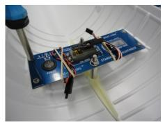
Now is a good time to mark and drill the servo screw holes into the crossmember. Use a 5/64" (2mm) drill for this kit's servo screws. READ THE WARNINGS on the crossmember when drilling holes or enlarging openings. Secure any loose wires on the Crossmember. TEMPORARILY install the crossmember with mounting screws. **ADVANCED:** Now is a good time to check the alignment of the keel to the rudder shaft if you want to do this.
