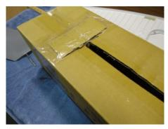
**Build a temporary Building Stand for the Keel.** Get or make a box at least 6 inches high, 5 inches wide and 12 inches long. Lay your Keel on it to mark where the upper leading edge of the Keel intersects the top and the rear bottom is even with the end of the box. Cut a 1/2-inch slot in the top to that point. In this box it was 10 inches. The length of the slpot depends on the height of the box.
