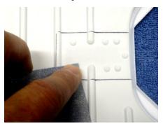
After the Mast Step Backer is glued in place, the Upper King Post Mount is glued over it on the underside of the deck. Set the mount in place and mark its outline on the underside of the Deck. Now sand this area. OK to sand the bumps.
