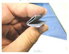
Firmly pinch the piece of Sandpaper over the top edge of the Hull and slide back and forth to roughen the surface. Open the piece and remove plastic debris often. The horizontal scratches will help the sealant grip the plastic. Sand half of the hull then refold the piece to sand the other half. Cut another piece about 1-1/2-inch square. Fold in half then fold again. Press tight.
