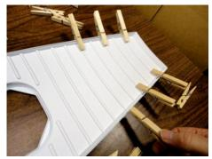
Center the tip of the Deck Liner to the tip of the Deck. Clamp 4 clothespins to the 2nd & 3rd ribs as shown. Check that the cockpit opening is still centered. Starting at the stern end, alternating left then right, attach clothespins to every other rib working toward the cockpit.
