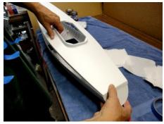
This bead of sealant will work. It is continuous with no gaps. It is just below the height of the Liner's side of the groove and about halfway up the edge of the Deck. In preparation to attach the Deck to the Hull, have 5 or 6 pre-cut pieces of tape nearby. Remember to tape down any loose wires in the deck. As before, engage the Transom first while holding up the other end of the Deck.
