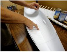
You can tape them in place. **Practice** setting the Hull Reinforcing Liner into the hull without touching the sides to prevent epoxy from rubbing off onto the hull. Repeat centering on the two locator bumps with your fingers and confirm the location with the end-marks you drew on the hull. The Hull should be sitting directly on the work table. To keep it from falling over, steady the sides with a folded towel or other object that won't get in the way of clamping.
