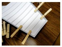
Carefully set the Deck Liner epoxy-side down into the Deck. Press the four corners of the cockpit opening to align it. Clamp 4 clothespins to the stern-end sides of the deck at these two ribs.
