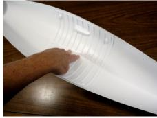
Inside the Hull at the center bottom where the Keel is installed you will see two locator points. The Hull Liner has two corresponding points. Using 2 fingers, slide the Hull Liner along the Hull until you feel the bumps line up. The bow-end of the Hull Liner is narrower than the stern and must be oriented to the bow of the Hull as shown.
