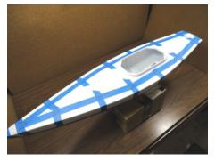
Keep working around the boat until everything is aligned. No additional tape is necessary. Before sealing up your tube of polyurethane sealant, run out several 3/16-inch diameter beads of sealant 6 to 8 inches long onto a plastic bag and mark the date on the bag. Store the beads of caulk with the Hull as it cures. To test the strength of the cured sealant, remove one of the beads and pull & stretch it to get an idea of how much the sealant on the hull has cured at that time.
