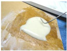
Sand the back of the ledge as well. Sand the **underside** of the Cockpit Cover in the same area. Mix two 1-inch circles of epoxy and add the same volume of filler. Put a 1/4-inch bend on the end of a paperclip to distribute the filled epoxy.
