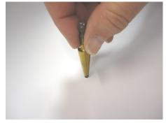
Clean off old Sharpie markings with alcohol. Locate the 3/16-inch point on the drill and mark that section plainly with the Sharpie marker. Drill the Rudder hole to a 3/16-inch diameter. By hand, you can use the step drill to de-burr the hole on the inside.
