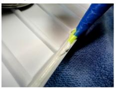
Don't try to do this in a continuous movement. A "stitching" move where you stop, letting the sealant build up then back up a fraction of an inch and let it fill again works well. High spots will happen. They can be scraped out later before you bond the Deck to the Hull. No hurry, take as long as you need. If sealant starts oozing out of a hole in the tape you may need to tape over or make a new nozzle and start again.
