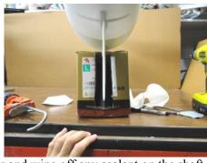
Once you are sure that the Rudder Mount brass tube is in the hole, remove the rudder and wipe off any sealant on the shaft. Clean with mineral spirits if necessary. The end of the brass tube should be even with the Hull as viewed from underneath. Re-insert the clean rudder shaft and clip the Safety Clip to the top to help hold the rudder mount in place. Use a paper towel to wipe off any excess sealant on the bottom of the hull. Wipe up any excess sealant around the Mount. Visually confirm the
