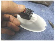
Take the pre-trimmed Rudder Servo Mount. Note the notch on the right side of the photo. That notch will engage the tip of the Rudder Mount. Note the rounded tunnel opening on the left. That is where your rudder wire will come out of the mount. Set the Rudder Servo mount into the hull with the notch touching the point on the Rudder Mount. Square the mount to the hull and trace its outline on the hull with a pencil. Sand the hull and the flange of the mount where they will be bonded. Use
