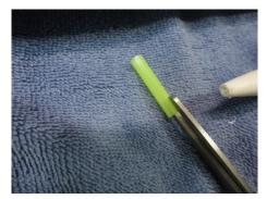
The nozzle of the tube of sealant is too large for the Deck groove. You need to extend the nozzle with a thin flexible tube.
