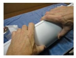
Tape the bow. The Hull should be in the groove of the Deck, but not fully seated. Using light pressure, push the Deck onto the Hull until you are at the indicator line you drew earlier.
