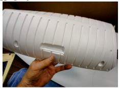
In the Hull Liner you will need to glue inserts into the two shelves that support the Crossmember and the two marked Anchor Points. Sand the 4 reinforcements and separate them from each-other. Each crossmember reinforcement is different.
