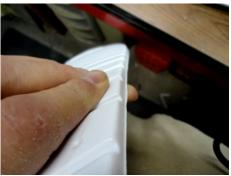
Lay out a towel & turn over the deck onto the towel. Sand the UNDERSIDE of the Deck thoroughly. Use a crisscross or circular pattern to roughen the surface for the epoxy to bond well. Sand the TOP of the Deck Reinforcing Liner. Check the edge trim of the Deck Liner. Use the sandpaper to straighten any uneven spots like at my thumb.
