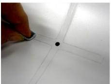
Insert the Rudder Mount into the hole with the **pointed end toward the Crossmember.** Align the point to the middle of the pencil line. Remove the Rudder Mount and sand the marked area. Also sand the corresponding bottom of the Rudder Mount.
