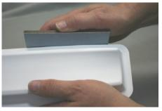
Bending down at the score will break the plastic along the scored line. Then, bend up to separate it cleanly. Don't tear or it will leave an uneven edge. You can cut with scissors if you prefer. Either way, any rough edges can be smoothed out with the included 100 grit sand paper.
