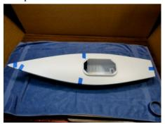
Working from the stern to the bow, tuck the Hull into the groove of the Deck. Add tape at the middle when you are farther along. When you finish a the tip of the bow, add a piece of tape there. Press evenly to ensure the deck is fully engaged onto the hull. Adjust the tape to remove any slack. No need to tightly pull the tape. It is just there to hold thing in place.
