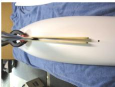
I flipped over the hull for clarity. You can do this with the Keel in the Keel Box as long as there is room for the sticks and clamp between the box top and the Hull. Paint stick or two rulers are clamped on the flat part of the Keel. The two sticks should be approximately centered on the hole for the rudder shaft. If not, the Keel holes can be adjusted to align before sealing the Keel Mount. After sealant is added but before the keel bolts are tightened, you can check again if needed.
