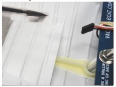
Press into place. Wipe away any excess sealant. Set the pre-trimmed Battery Tray into the Bow. It only fits into this location. Trace its outline onto the hull with a pencil. Sand the Tray and Hull at the point of contact. If you plan to put a strip of Velcro® on the battery tray, do it now, before you apply sealant or do it tomorrow after the sealant has cured some and before you install the Deck.
