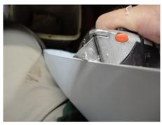
Smooth any high spots. Use the sandpaper or lightly scrape with a knife. The sealant used in attaching the deck will bridge any low spots so it does not have to be perfect. Note the Transom has a curved top to match the crown of the deck.
