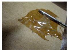
Lay out the shelf inserts and anchor point inserts near where they go to avoid mistakes. Pour two 1-1/4-inch circles of 30 minute epoxy and mix. A steel rod works well for this. A 1/8" diameter rod was used for these photos.
