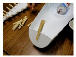
Don't forget the sides. Insert the Transom Reinforcement into the Transom, pressing it into place while supporting the outside of the Transom. Clamp one clothespin fully onto the Transom center. Check the alignment.
