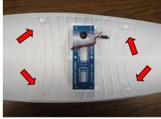
Use a pencil to mark the edges of the Hull Liner onto the hull. This will help you align it later and marks the area on the Hull you will need to sand. The Crossmember looks like this. Bow is on the right. Note the 4 bumps on the Hull Liner. These are possible anchor points if your rigging requires them. Mark the two you plan to use. Your rig may not require internal anchor points. External anchor points up on the deck can make rigging adjustments much easier.
