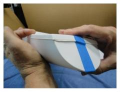
Move along seating the Deck over the Hull. As you seat the Deck, re-position the tape. No need to pull hard. The sealant will stay in place. The tape just holds it there. There will be lots of oozing at the Transom. Once the Deck is on the line, add tape to the sides of the stern of the boat.
