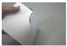
Styrene can be cut by scoring and breaking, or with scissors. The first score should be very light while concentrating on accuracy. The second and third score is made with more pressure and will follow the first. Repeat scoring the line until the part separates or after 2 or 3 scores, bend the plastic to break it.
