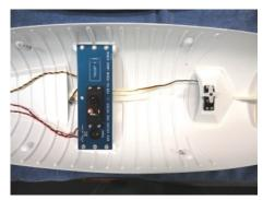
Run the double folded sandpaper back and forth in the grooves of the Deck. **Remove it often** to clean off any plastic debris. Check it for loss of granules and refold as needed to finish the job. Now is a good time to install any equipment you plan to use in the boat. Velcro® for the Battery Tray, wiring and Servo for the Crossmember and the Rudder Servo. Tape down any loose wires to keep them away from the Deck to Hull joint. No need to install the rudder or linkage at this time.
