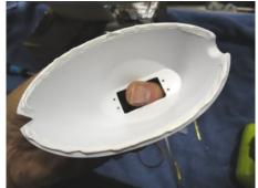
. Drill a 1/8-inch hole at each corner of your measurements and connect the holes by scoring through with a knife. Use the rudder servo to locate and drill its mounting holes with a 1/16" drill bit. Apply a thin bead of sealant and set the Rudder Servo Mount into the hull aligning it with the Rudder Mount and the pencil marks you made earlier.
