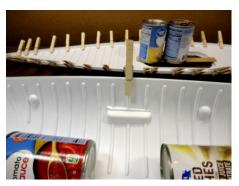
The cans will hold down the Hull Liner. You start clamping the top at the center. Lightly pinch the sides together with your left hand while you clamp with your right. Center the clothespin on the rib.
