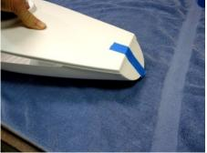
Because the Transom is angled, you have to engage the Deck into the Transom first, at an angle. Once the Deck in on the Transom, put a piece of masking tape over the end to hold it in place.
