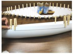
Support the edges in order to sand the sides evenly. In the Hull, mark the lines for the Hull Liner with 4 clothespins. On the outside of the Hull, center the Clamping Strip between those markers and clamp in place. The strips help prevent the clothespins from dimpling the sides of the hull.
