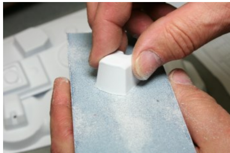
Sand on the sanding block. Rotate it frequently to keep the base of the gun square and even on all sides. Sand just until the rounded bottom is gone as shown on the right photo, “after” on left and “before” on right.
