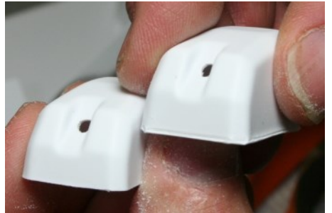
Sand on the sanding block. Rotate it frequently to keep the base of the gun square and even on all sides. Sand just until the rounded bottom is gone as shown on the right photo, “after” on left and “before” on right.
