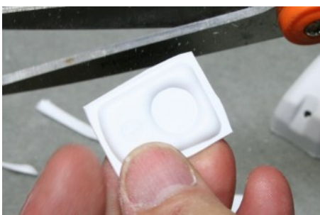
Now trimmed just outside of the raised rounded area, mark the outer edge of that raised area with a pencil to help locate the cut-line. Trim to the mark with scissors.
