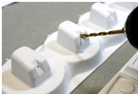
Before separating the 5-inch gun tops, choose the angle of your gun barrels. Put a dot on each cannon where you plan to drill. Hold the drill at the same angle for each cannon. Slowly drill a 1/8-inch hole in each cannon.
