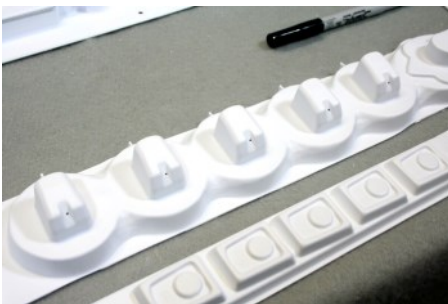
Before separating the 5-inch gun tops, choose the angle of your gun barrels. Put a dot on each cannon where you plan to drill. Hold the drill at the same angle for each cannon. Slowly drill a 1/8-inch hole in each cannon.
