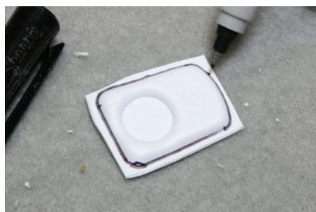
Now trimmed just outside of the raised rounded area, mark the outer edge of that raised area with a pencil to help locate the cut-line. Trim to the mark with scissors.
