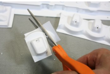
Gradually trim the plastic closer to the sides of a cannon. For your final cuts, lay the top blade of the scissors flat against the side you are trimming . Don't forget the 45 degree corner cuts on the front.
