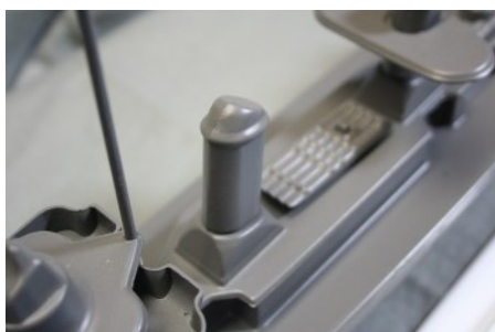
The stacks are formed in halves. They glue together and sit on the angled bases on the 2nd deck. The rear-most stack has a wing that mounts searchlights.
