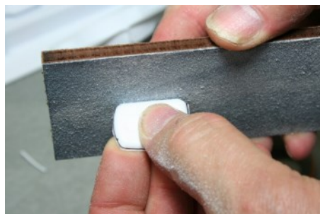
Cut the tiny 45 degree front angles and carefully trim the rounded back area. Sand the sides to make them even with the bottom of the round edge. Here are two halves of a gun ready to be glued together. If you are worried about a gun getting knocked off in a collision, put a small piece of Styrofoam inside the housing. 9
