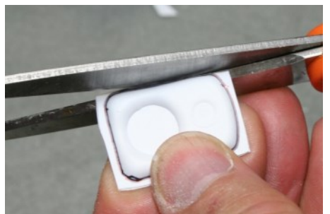
Now trimmed just outside of the raised rounded area, mark the outer edge of that raised area with a pencil to help locate the cut-line. Trim to the mark with scissors.
