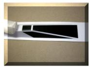
From the front, peel the application tape off of the decal. Peel slowly, making sure that you are not lifting off the decal at the same time.
