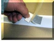
When it is aligned, press across the front and begin to peel the backing paper off.
